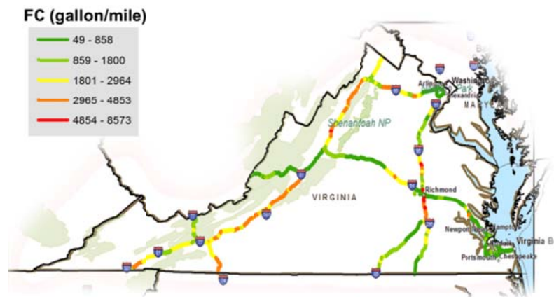
Figure 7: Annual excess fuel consumption per mile due to deflection and roughness induced PVI of trucks on Virginia’s interstate system. Roughness data are from 2013 and deflection data are from 2007.
